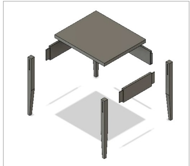
John Moussa yr 12 Industrial technology Fusion 365 drawing of table components and joints.
